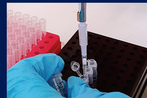
The test uses a simple colour change to identify presence of the virus. Positive samples change from pink to yellow. Each test uses three vials, each with different primers. A positive test would turn two samples pink, and leave one yellow as a negative control to confirm the test is working.
